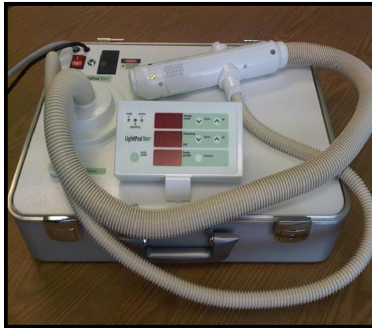
**Figure 2. Nd:YAG 1064nm Laser.**
